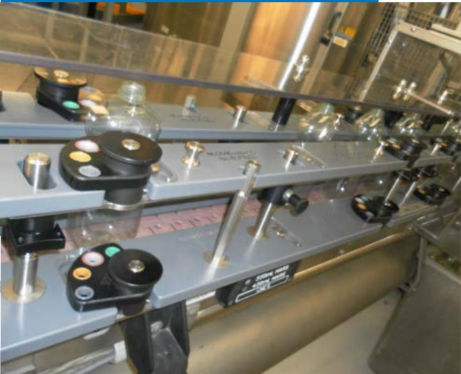
Similar to our other parts these conveyor guiderails are generally manufactured in 316 stainless steel and UHMWpe and are custom designed to suit specific containers.
